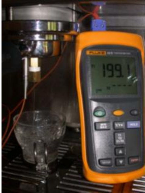
Figure. 3 Installed portafilter thermometer measuring the temperature of the metered brew water stream.
