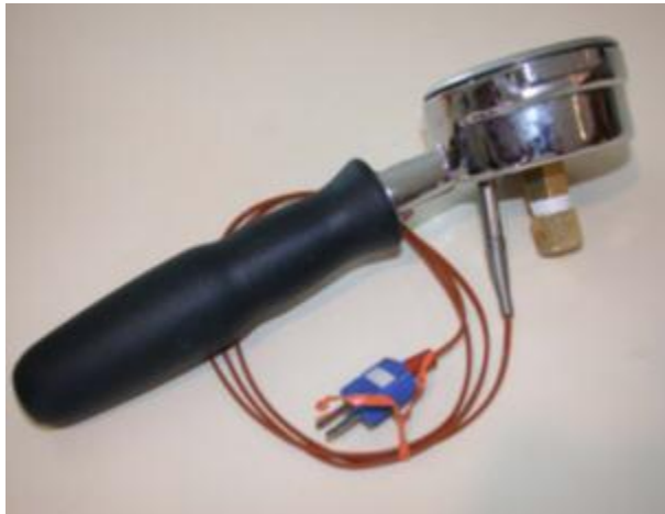
Figure. 2 Portafilter thermometer side view, showing the thermocouple probe's exit through the bottom of the portafilter, and the brew water metering orifice.
