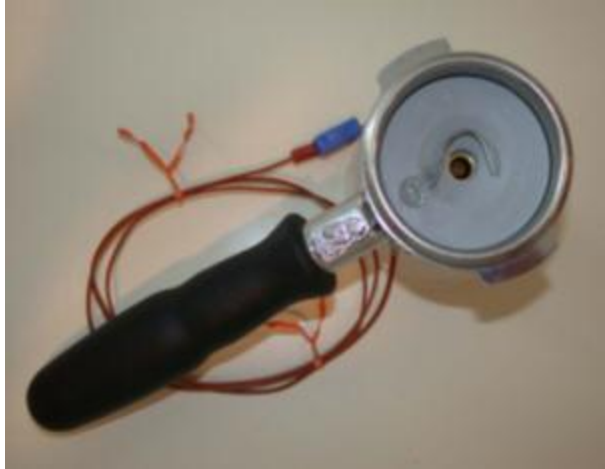
Figure. 1 Portafilter thermometer top view, showing the Type T thermocouple probe and the coffee cake facsimile.
